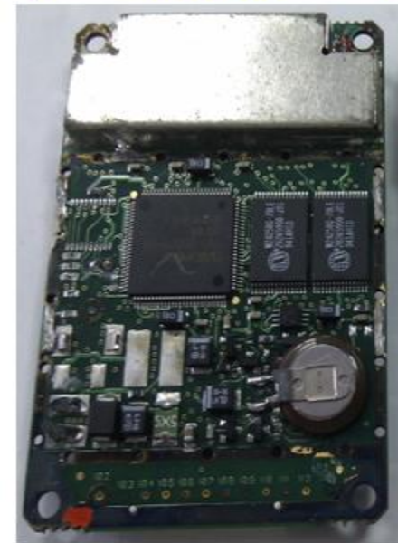
After Gold stripping
